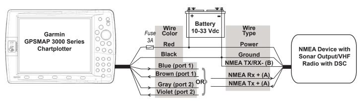
GPSMAP 3000 Series Chartplotter Wired to a NMEA Device With Two-way Communication
