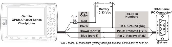
GPSMAP 3000 Series Chartplotter Wired to a DB-9 Serial PC Connector
